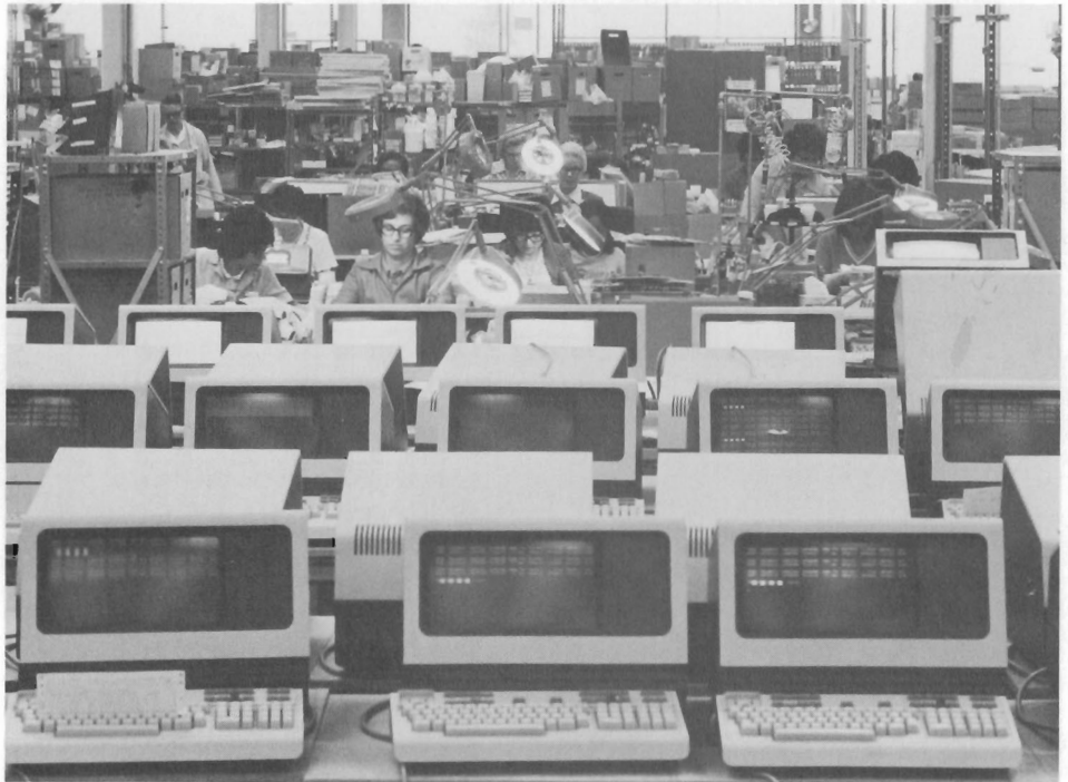
Lines of CRT terminals blink their way through self-testing as HP people touch-up PC boards in the terminal production area in Cupertino. HP has shipped more than 2,000 units since deliveries began early this year.
